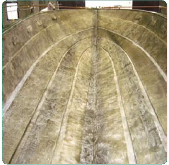
Fig. 4 – The fully-cured skin coat.
