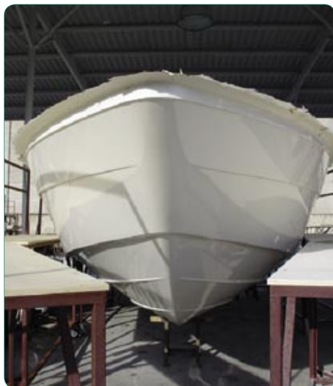
Fig. 11 – The hull following demolding.
