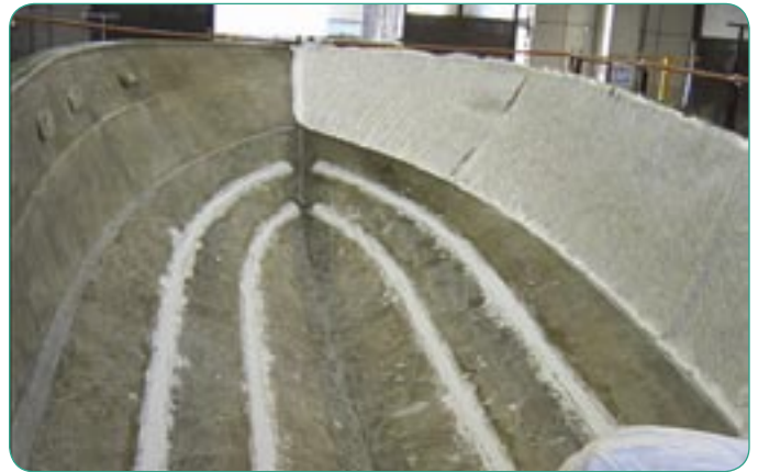
Fig. 5 - Levelling the spray rails.
