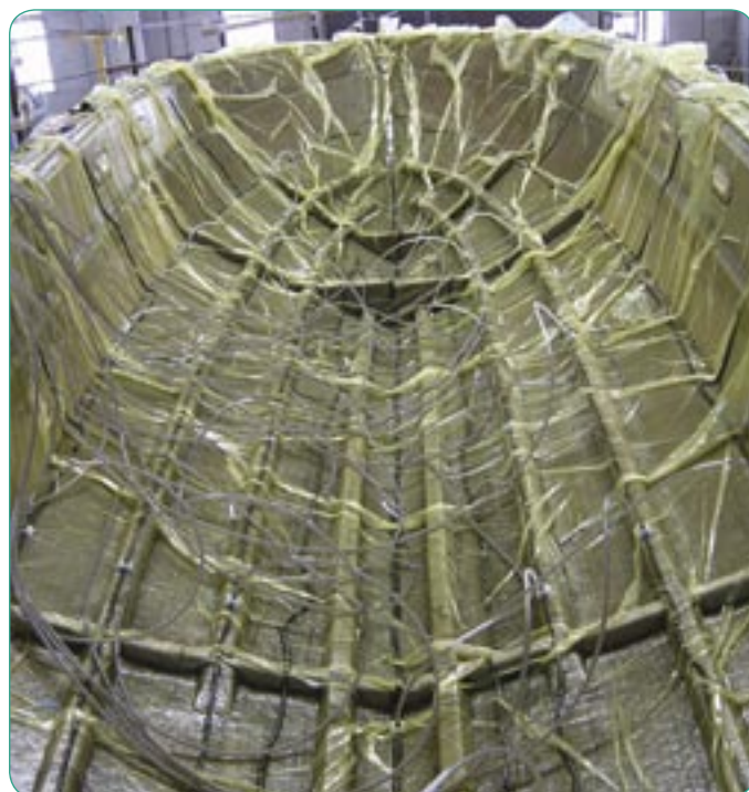
Fig. 15 - 3-D infusion of a 38 feet hull.
